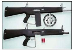
The plastic and aircraft steel construction functions without lubrication and cleaning, and can fire with a 300rpm rate of fire. It can also use the new FRAG-12 round, a high-explosive round which will blow a one-inch hole in steel plate and up to four inches of aluminum plating, and also create a two-meter casualty radius.
